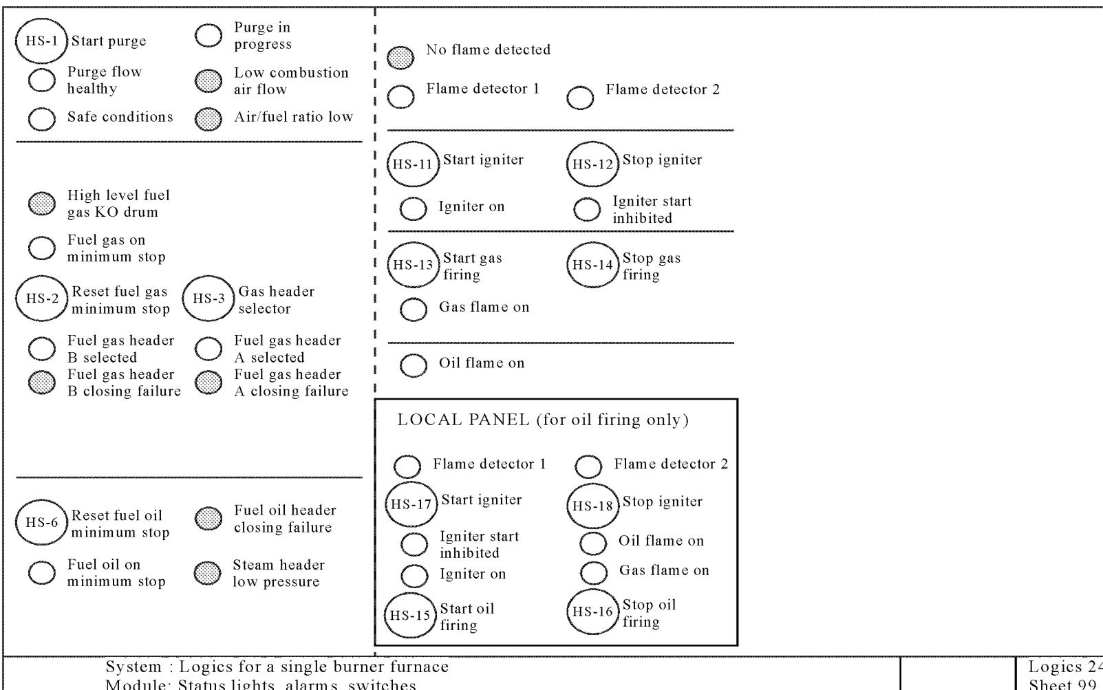
System : Logics for a single burner furnace
